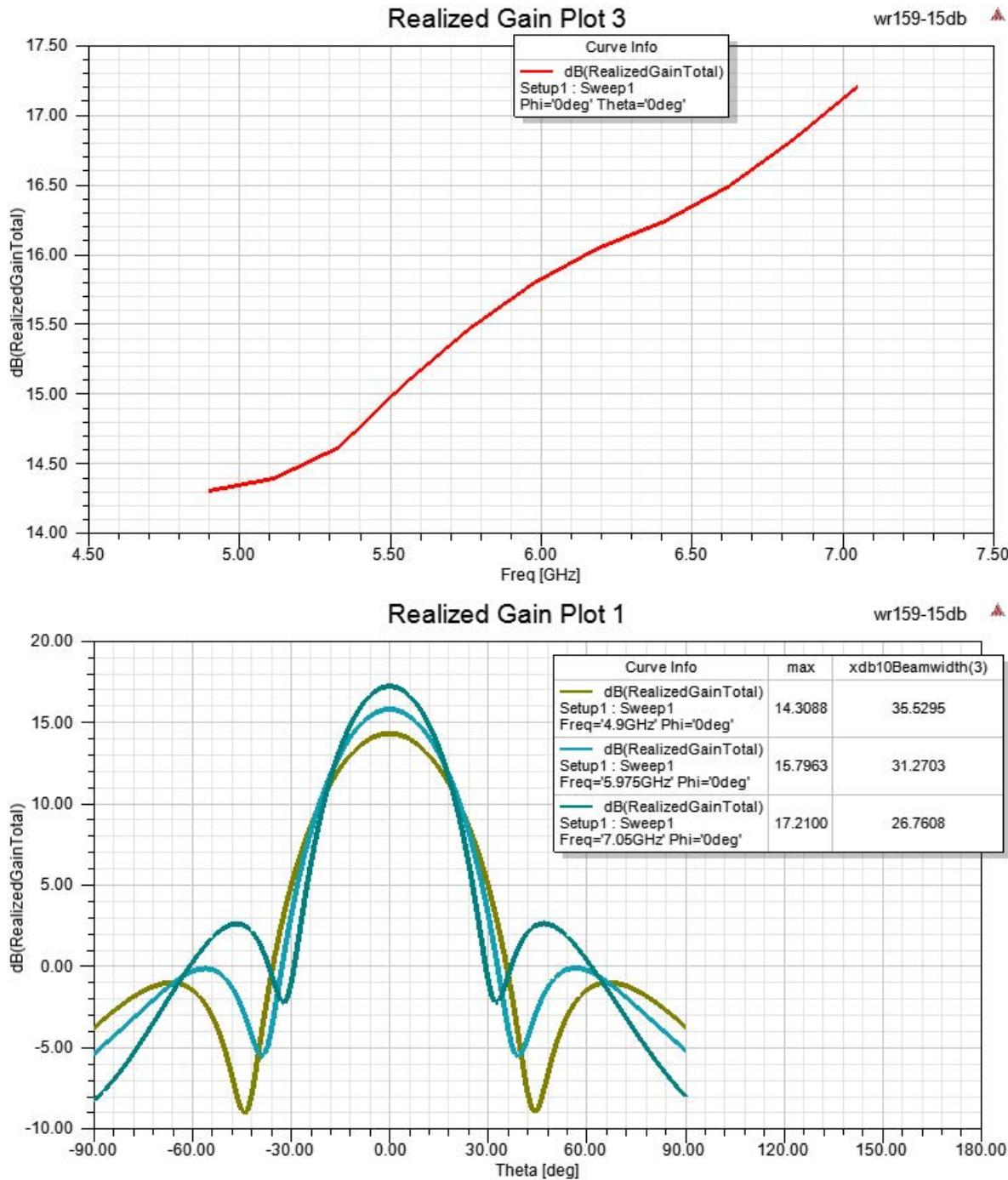
WR-159 Standard Gain Horn with 15 dBi gain, N Female Connector, Integrated Cage-Style Mount
