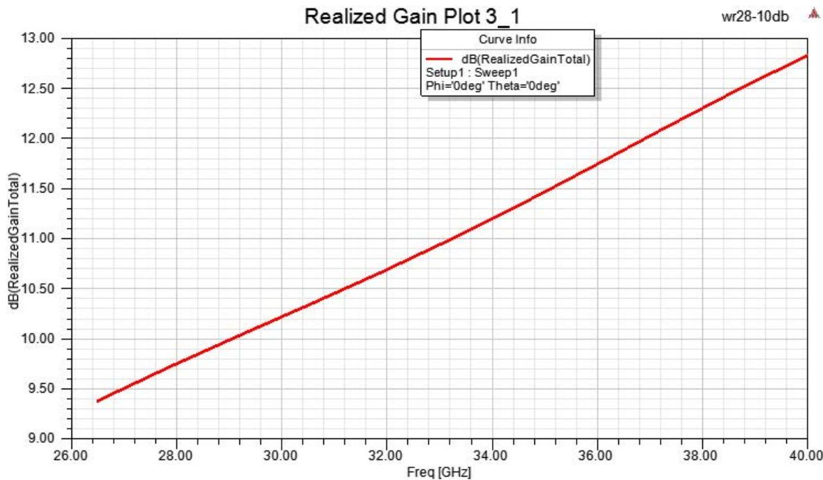
WR-28 Standard Gain Horn with 10 dBi gain, 2.92mm
