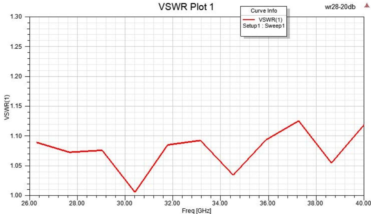
WR-28 Waveguide Antenna, 26.5 GHz to 40 GHz Frequency Range, 20 dBi Gain, UG-599/U Flange with Pre-Installed L mount
