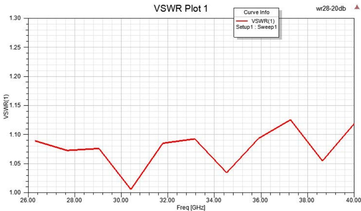
WR-28 Standard Gain Horn with 20 dBi gain, 2.92mm
