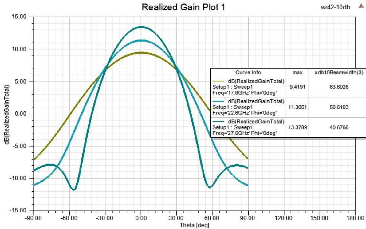
WR-42 Standard Gain Horn with 10 dBi gain, 2.92mm Female connector, with Pre-Installed L Mount
