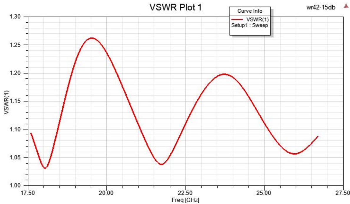
WR-42 Standard Gain Horn with 15 dBi gain, 2.92mm
