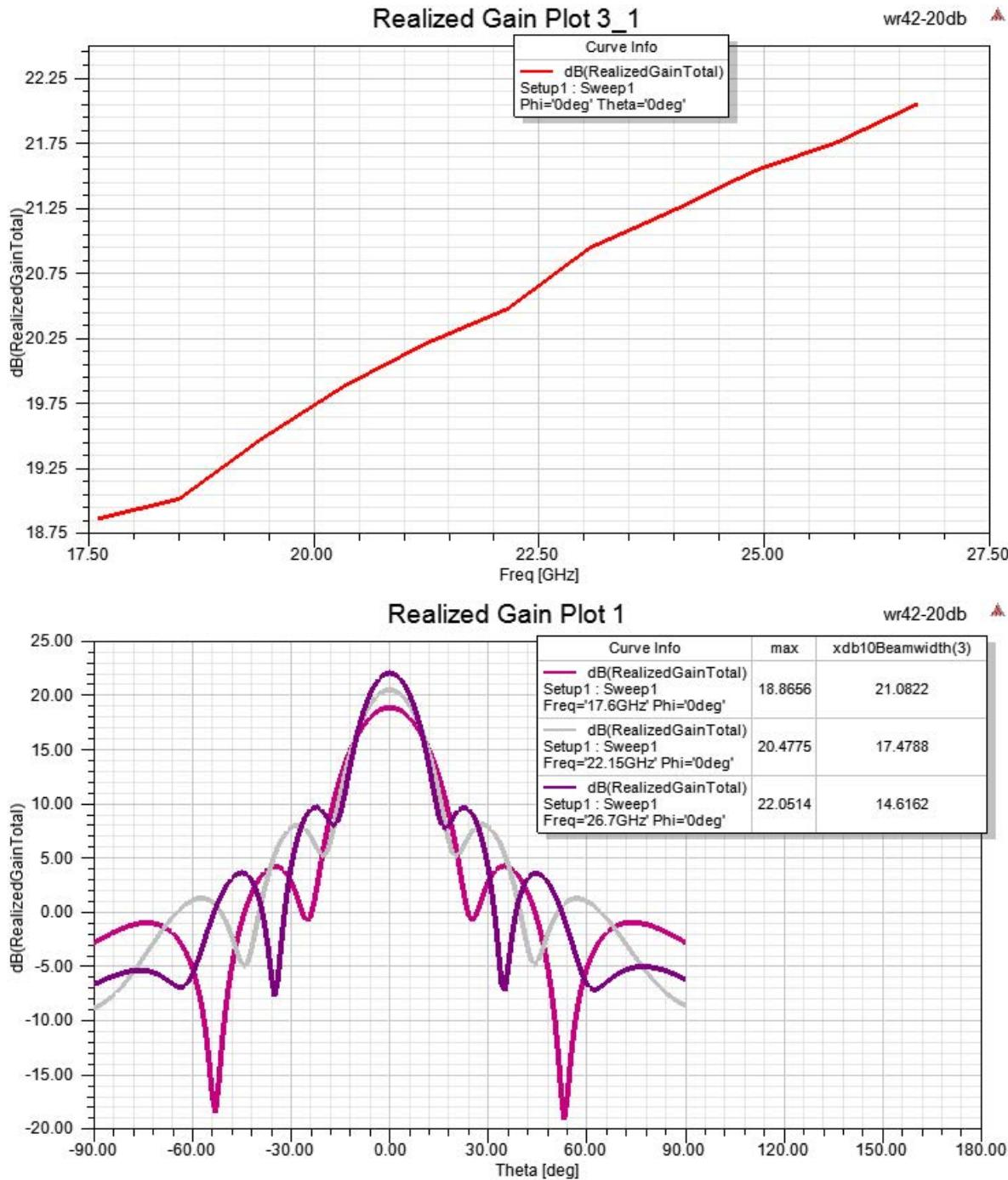
WR-42 Standard Gain Horn with 20 dBi gain, 2.92mm Female connector, with Pre-Installed L Mount
