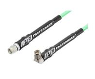
SMA Male to SMA Male Right Angle Low Loss Test Cable 36 Inch Length Using PE-P142LL Coax with HeatShrink, LF Solder
