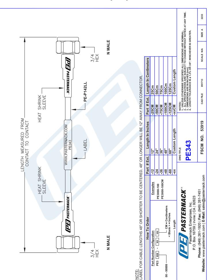
PE343-50CM CAD Drawing N Male to N Male Low Loss Test Cable 50 CM Length Using PE-P142LL Coax, RoHS
