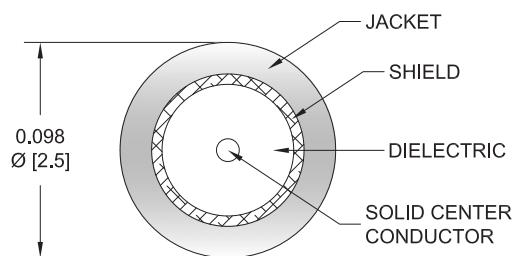
SMA Male to N Female Bulkhead Semi-Flexible Precision Cable 18 Inch Length Using PE-SR405FLJ Coax, RoHS
