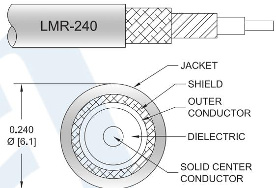
Click the following link (or enter part number in "SEARCH" on website) to obtain additional part information including price, inventory and certifications: [7/16 DIN Male Right Angle to 7/16 DIN Male Right Angle Low Loss Cable Using LMR-240 Coax with HeatShrink PE3C1064/HS](#)
