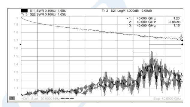
ELECTRICAL LENGTH (TWO WAY) = 5473PS ELECTRICAL LENGTH (ONE WAY) = 2736PS
