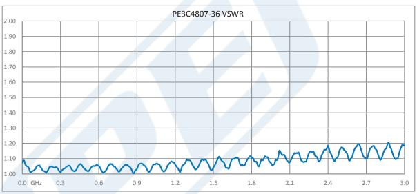
Click the following link (or enter part number in "SEARCH" on website) to obtain additional part information including price, inventory and certifications: Snap-On MMBX Plug Right Angle to SMA Female Bulkhead Cable 12 Inch Length Using RG178 Coax PE3C4807-12
