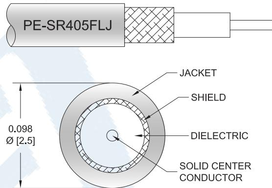
Click the following link (or enter part number in "SEARCH" on website) to obtain additional part information including price, inventory and certifications: [Slide-On BMA Jack 2 Hole Flange to SMA Male Right Angle Cable 6 Inch Length Using PE-SR405FLJ Coax PE3C4858-6](#)
