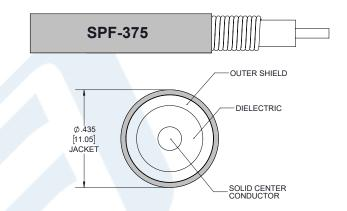
inventory and certifications: Fire Rated N Female to N Female Low PIM Cable Using SPF-375 Coax Using Times Microwave Parts PE3C6379
