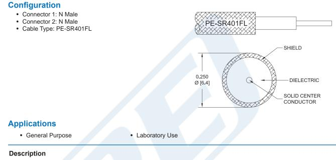
Pasternack's PE3W00109-24 type N male to type N male 24 inch cable using PE-SR401FL coax is part of our full line of RF components available for same-day shipping. Pasternack's formable RF cable assemblies provide an alternative to costly preformed semi-rigid assemblies since they are hand formable. This Pasternack type N to type N cable assembly has a male to male gender configuration with 50 ohm formable PE-SR401FL coax.
