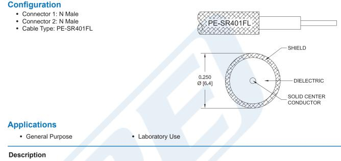
Pasternack's PE3W00109-36 type N male to type N male 36 inch cable using PE-SR401FL coax is part of our full line of RF components available for same-day shipping. Pasternack's formable RF cable assemblies provide an alternative to costly preformed semi-rigid assemblies since they are hand formable. This Pasternack type N to type N cable assembly has a male to male gender configuration with 50 ohm formable PE-SR401FL coax.
