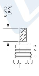
FORM BRAID OVER CLAMP NUT (4). TRIM BRAID BACK TO SHOULDER. CUT DIELECTRIC & CENTER CONDUCTOR TO DIMENSION SHOWN. DO NOT NICK CENTER CONDUCTOR. SOLDER CONTACT TO CENTER CONDUCTOR. REMOVE EXCESS SOLDER. CENTER CONDUCTOR. REMOVE EXCESS SOLDER. DO NOT OVER HEAT DIELECTRIC. INSERT CABLE ASSEMBLY INTO BODY & TIGHTEN. ς.
