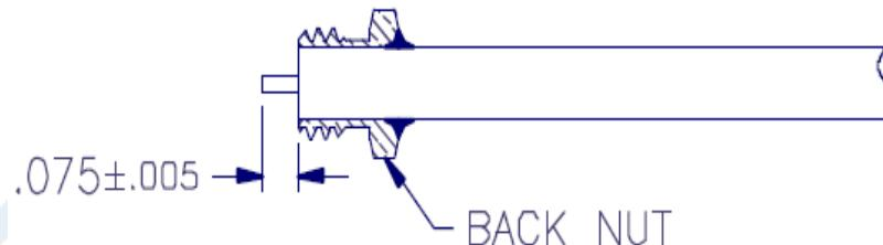
2. SLIDE BACK NUT ONTO CABLE UNTIL TRIMMED END OF JACKET IS FLUSH WITH FRONT OF NUT. SOLDER NUT TO CABLE.
