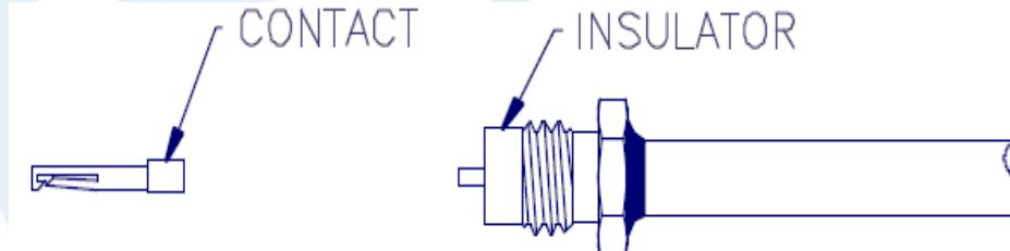
4. INSTALL INSULATOR OVER CABLE CENTER CONDUCTOR.
