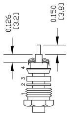
NOTE: RG62 USES PTFE INSERT. INSERT PTFE BEFORE CONTACT. TAPER END FIRST.
