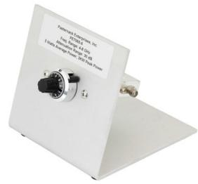
0 to 30 dB Rotary Continuously Variable Attenuator, SMA Female To SMA Female Rated To 5 Watts From 4 GHz To 8 GHz from Pasternack Enterprises has same day shipment for domestic and International orders. Our RF, microwave and millimeter wave products maintain a 99.4% availability and are part of the broadest selection in the industry.
