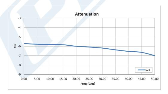
Click the following link (or enter part number in "SEARCH" on website) to obtain additional part information including price, inventory and certifications: 6 dB Fixed Attenuator, 2.4mm Male to 2.4mm Female Passivated Stainless Steel Body Rated to 1 Watt Up to 50 GHz PE7089-6
