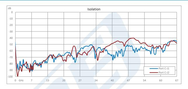
Click the following link (or enter part number in "SEARCH" on website) to obtain additional part information including price, inventory and certifications: Absorptive SPDT PIN Diode Switch Operating from 100 MHz to 67 GHz Up to 0.5 Watts (+27 dBm) and 1.85mm PE71S2050
