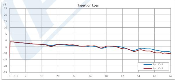
Click the following link (or enter part number in "SEARCH" on website) to obtain additional part information including price, inventory and certifications: Absorptive SPDT PIN Diode Switch Operating from 100 MHz to 67 GHz Up to 0.5 Watts (+27 dBm) and 1.85mm PE71S2050
