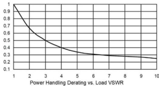
Power handling chart and derating curves based on the following conditions:
