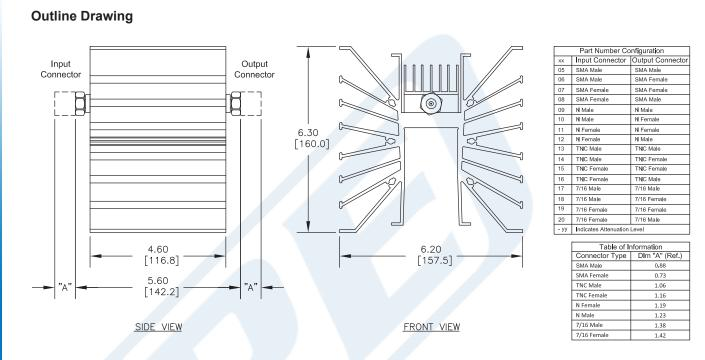
30 dB Fixed Attenuator, TNC Male To TNC Female Directional Black Aluminum Heatsink Body Rated To 300 Watts Up To 3 GHz from Pasternack Enterprises has same day shipment for domestic and International orders. Our RF, microwave and millimeter wave products maintain a 99% availability and are part of the broadest selection in the industry.
