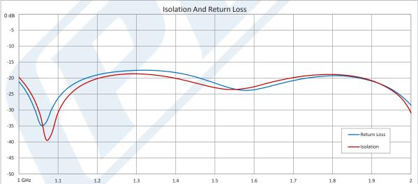
Click the following link (or enter part number in "SEARCH" on website) to obtain additional part information including price, inventory and certifications: High Power Isolator with 18 dB Isolation from 1 GHz to 2 GHz, 100 Watts and SMA Female PE83IR1000
