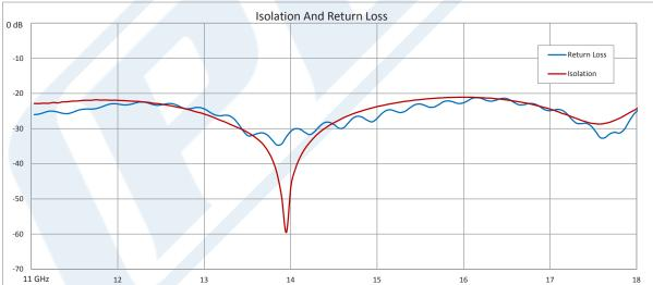
Click the following link (or enter part number in "SEARCH" on website) to obtain additional part information including price, inventory and certifications: High Power Isolator With 20 dB Isolation From 11 GHz to 18 GHz, 50 Watts And SMA Female PE83IR1011
