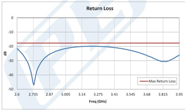
Click the following link (or enter part number in "SEARCH" on website) to obtain additional part information including price, inventory and certifications: WR-284 CPR-284G Grooved Flange to N Female Waveguide to Coax Adapter Operating From 2.6 GHz to 3.95 GHz, S Band PE9842
