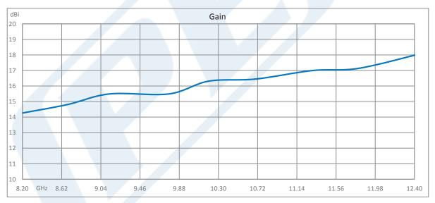
Click the following link (or enter part number in "SEARCH" on website) to obtain additional part information including price, inventory and certifications: WR-90 Waveguide Standard Gain Horn Antenna Operating From 8.2 GHz to 12.4 GHz With a Nominal 15 dBi Gain With UG-135/U Square Cover Flange PE9856-15
