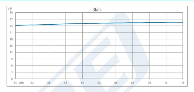
WR-15 Waveguide Standard Gain Horn Antenna Operating from 50 GHz to 75 GHz with a Nominal 25 dBi Gain with UG-385/U-Mod Round Cover Flange from Pasternack Enterprises has same day shipment for domestic and International orders. Our RF, microwave and millimeter wave products maintain a 99.4% availability and are part of the broadest selection in the industry.
