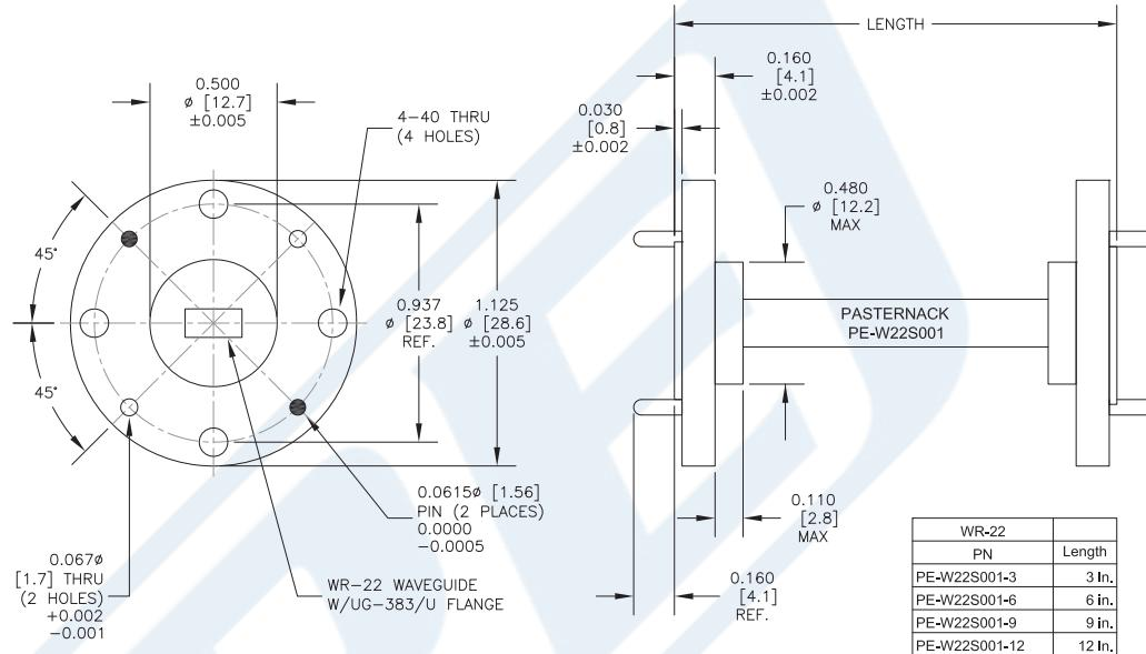
WR-22 Instrumentation Grade Straight Waveguide Section 12 Inch Length with UG-383/U Flange Operating from 33 GHz to 50 GHz from Pasternack Enterprises has same day shipment for domestic and International orders. Our RF, microwave and millimeter wave products maintain a 99% availability and are part of the broadest selection in the industry.
