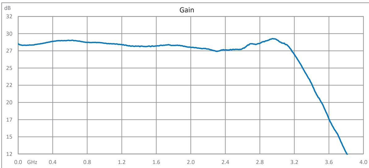
1 Watt P1dB, 30 MHz to 3 GHz, Medium Power GaAs
