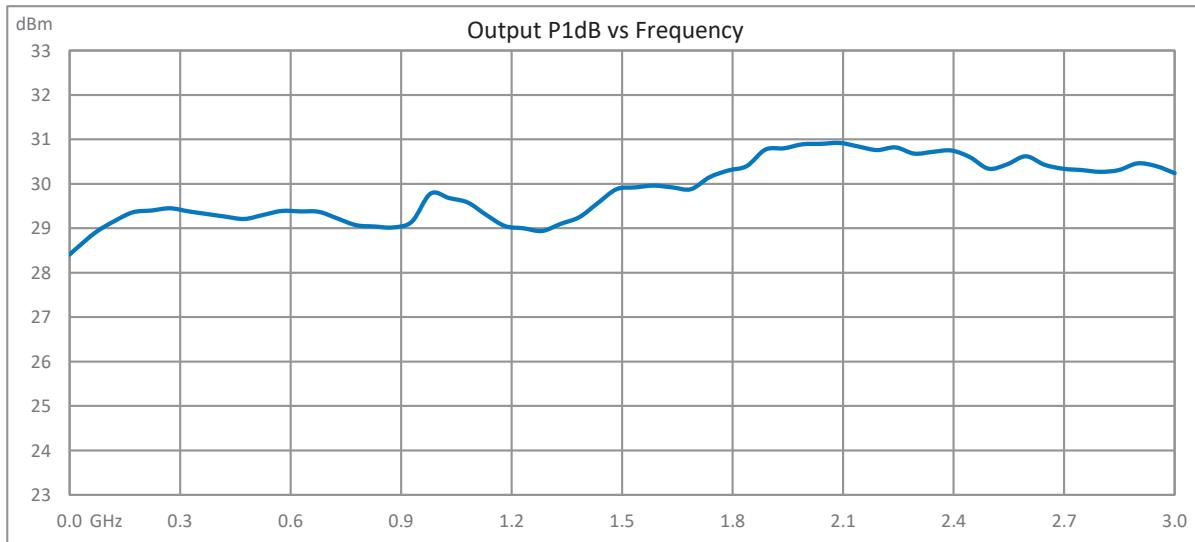
1 Watt P1dB, 30 MHz to 3 GHz, Medium Power GaAs Amplifier, SMA Input, SMA Output, 27 dB Gain, 39 dBm IP3 from Pasternack Enterprises has same day shipment for domestic and International orders. Our RF, microwave and millimeter wave products maintain a 99.4% availability and are part of the broadest selection in the industry.
