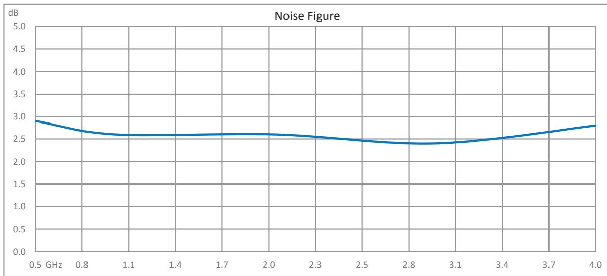
1 Watt P1dB, 500 MHz to 4 GHz, Medium Power Amplifier with Heatsink, SMA, 30 dB Gain, 6 dB NF
