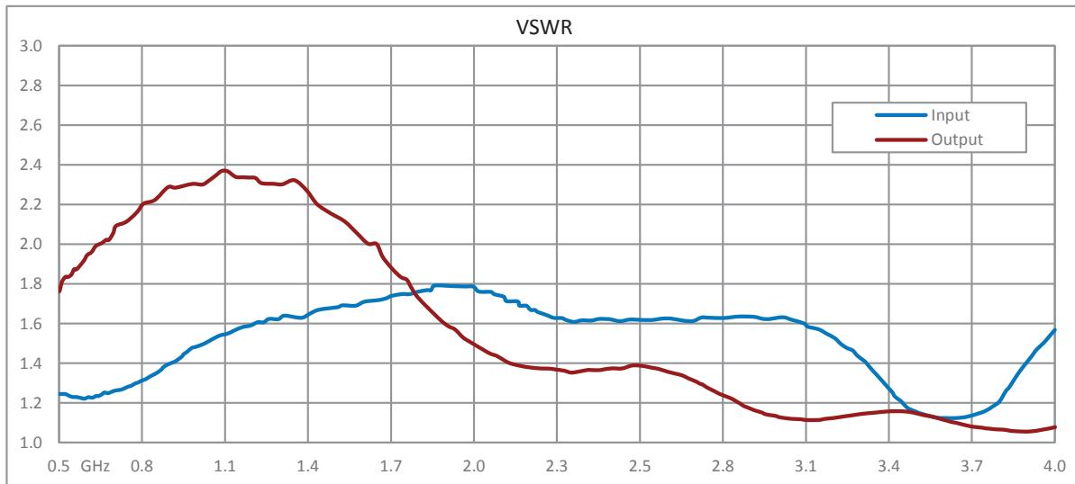
1 Watt P1dB, 500 MHz to 4 GHz, Medium Power
