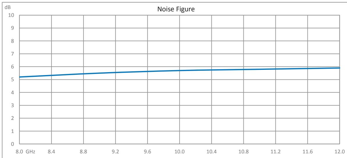
5 Watt P1dB, 8 GHz to 12 GHz, High Power Amplifier
