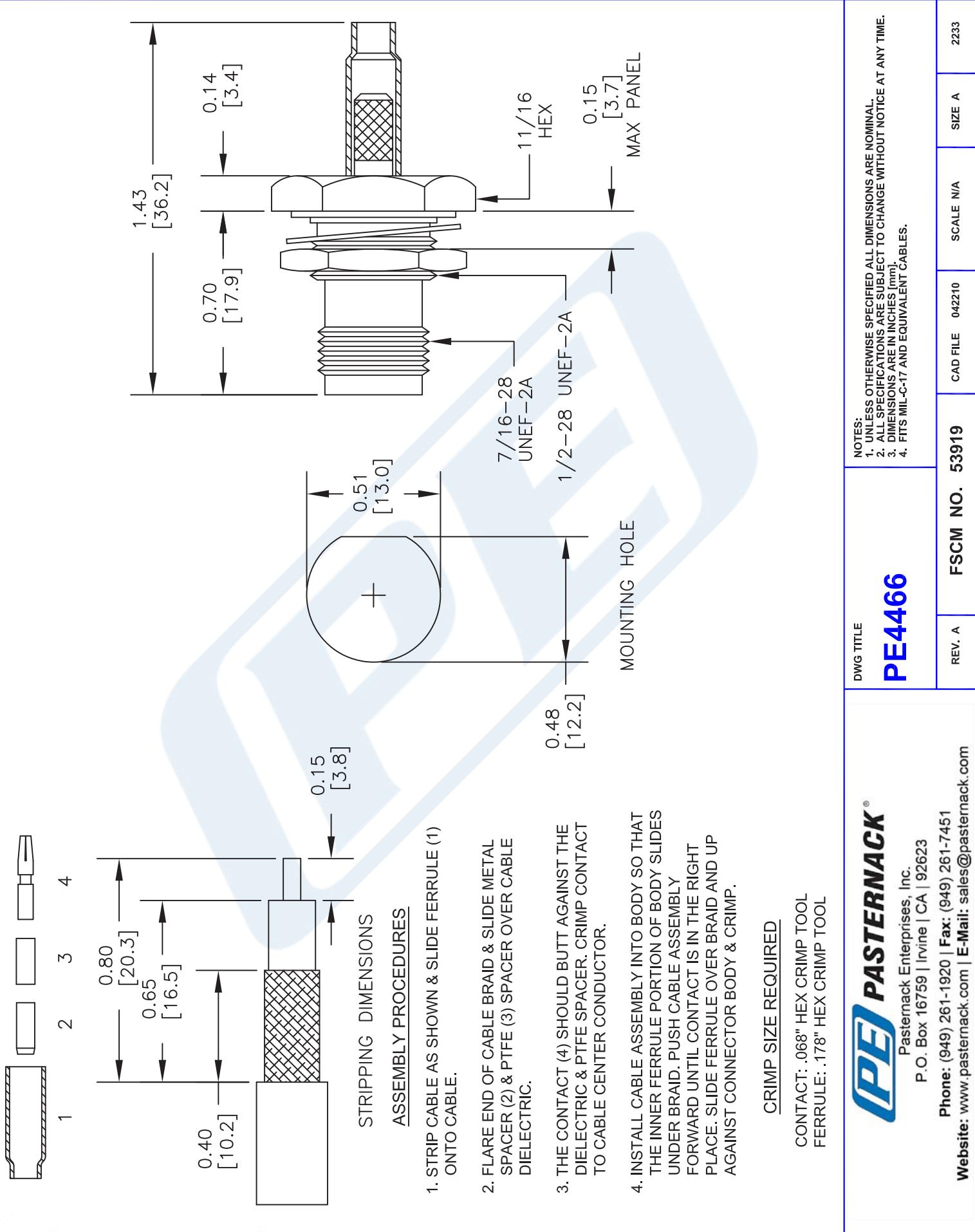
MMCX Plug Right Angle Connector Crimp/Solder Attachment for RG174, RG316, RG188, LMR-100, PE-B100, PE-C100, 0.100 inch
