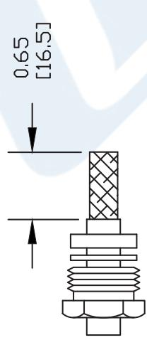
2. FORM BRAID OVER CLAMP NUT (4). TRIM BRAID BACK TO SHOULDER. CUT DIELECTRIC & CENTER CONDUCTOR TO DIMENSION SHOWN. DO NOT NICK CENTER CONDUCTOR. TIN CENTER CONDUCTOR SLIDE ASSEMBLY INTO BODY, SOLDER CENTER CONDUCTOR IN PLACE, TIGHTEN CLAMP NUT & SCREW CAP
