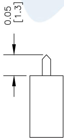
2. INSERT CABLE AND CONTACT INTO CONNECTOR BODY UNTIL FULLY ENGAGED. SOLDER BODY TO CABLE.
