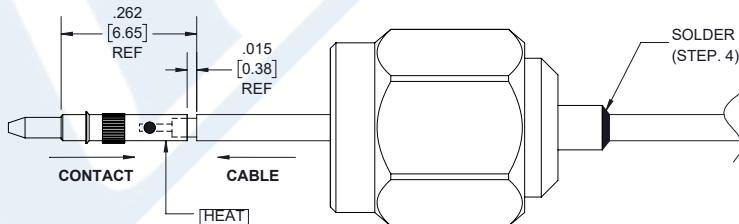
4. USING ASSEMBLY TOOL, PRESS CONTACT FULLY INTO INSULATOR. SOLDER OUTER CONDUCTOR TO BODY.
