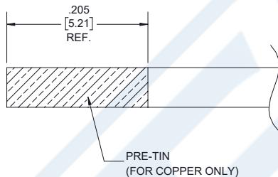
2. A. STRIP CABLE TO THE DIMENSIONS AS SHOWN TO EXPOSE CENTER CONDUCTOR AND DIELECTRIC.
