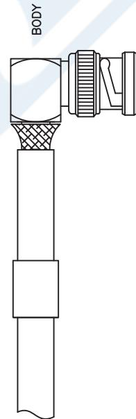
3. SLIDE FERRULE OVER BRAID UP TO THE CONNECTOR BODY AND CRIMP AS CLOSE TO THE CONNECTOR BODY AS POSSIBLE USING A .255" HEX CRIMP TOOL.
