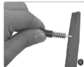
Chamfer inner conductor 0.5 × 45° with flat file.
