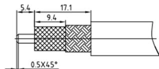
1.A. Stripping dimension is as shown by diagram, attention should be paid while stripping.
