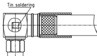
2.A. Put the connector in place, Then push the ferrule.
