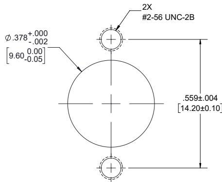
Slide-On BMA Jack 2 Hole Flange to Slide-On BMA Jack
