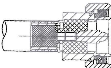
3. A. Insert Cable into connector body until dielectric is seated and center conductor is inserted fully into connector center pin.
