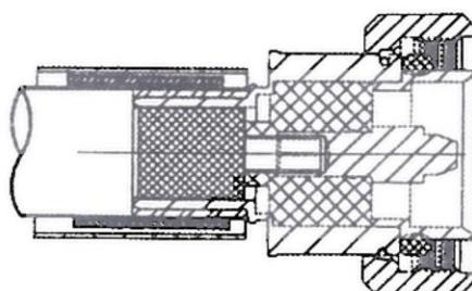
4. A. Slide crimp ferrule over braid and crimp as close to body as possible using .429" HEX crimp tooling
