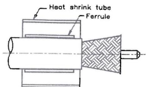
2. A. Slide crimp ferrule and heat shrink tube over the cable
