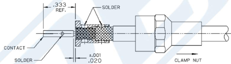
3. INSERT CABLE/CONTACT SUB-ASSEMBLY INTO CONNECTOR UNTIL SEATED AND TIGHTEN CLAMP NUT TO 35-45 IN-LBS.
