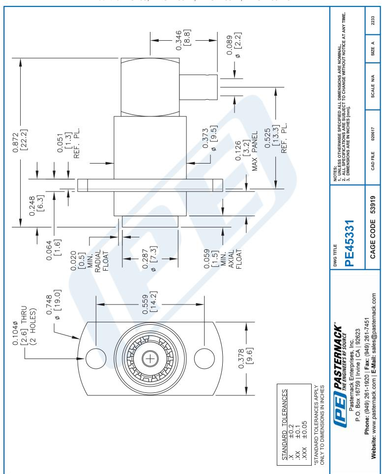
BMA Jack Right Angle Slide-On Connector Solder Attachment 2 Hole Flange Mount for RG405, PE-SR405AL, PE-SR405FL, PE-SR405FLJ
