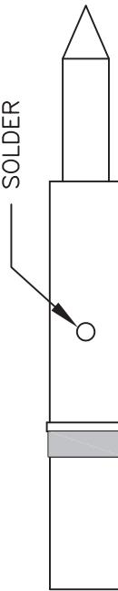
3. SLIDE INSULATOR THROUGH CONTACT UNTIL IT BOTTOMS OUT. INSERT INSULATOR TO BODY UNTIL IT MATES. SOLDER BODY TO CABLE.
