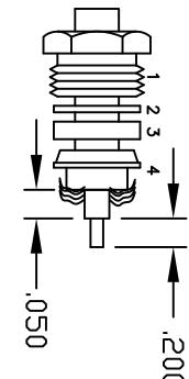
NOTE: INSERT PTFE BEFORE CONTACT. WITH LARGE OPEN END SLIDING OVER CENTER CONDUCTOR & DIELECTRIC.
