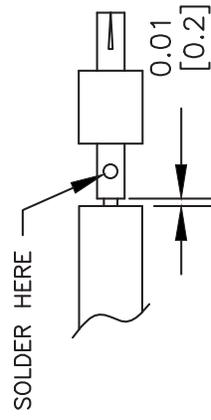
3. INSERT CABLE FULLY INTO BODY. SOLDER OUTER CONDUCTOR TO BODY.
