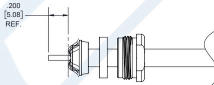
3. SLIDE WASHER (4) AND HALF-INSULATOR (5) AGAINST THE BRAID CLAMP AND HOLD BRAID IN PLACE. SOLDER CONTACT (6) TO CENTER CONDUCTOR. REMOVE EXCESS SOLDER. DO NOT OVER HEAT DIELECTRIC. SLIDE A REST HALF-INSULATOR (5) TO LOCKED CONTACT. INSERT CABLE ASSEMBLY INTO BODY (7) & TIGHTEN.
